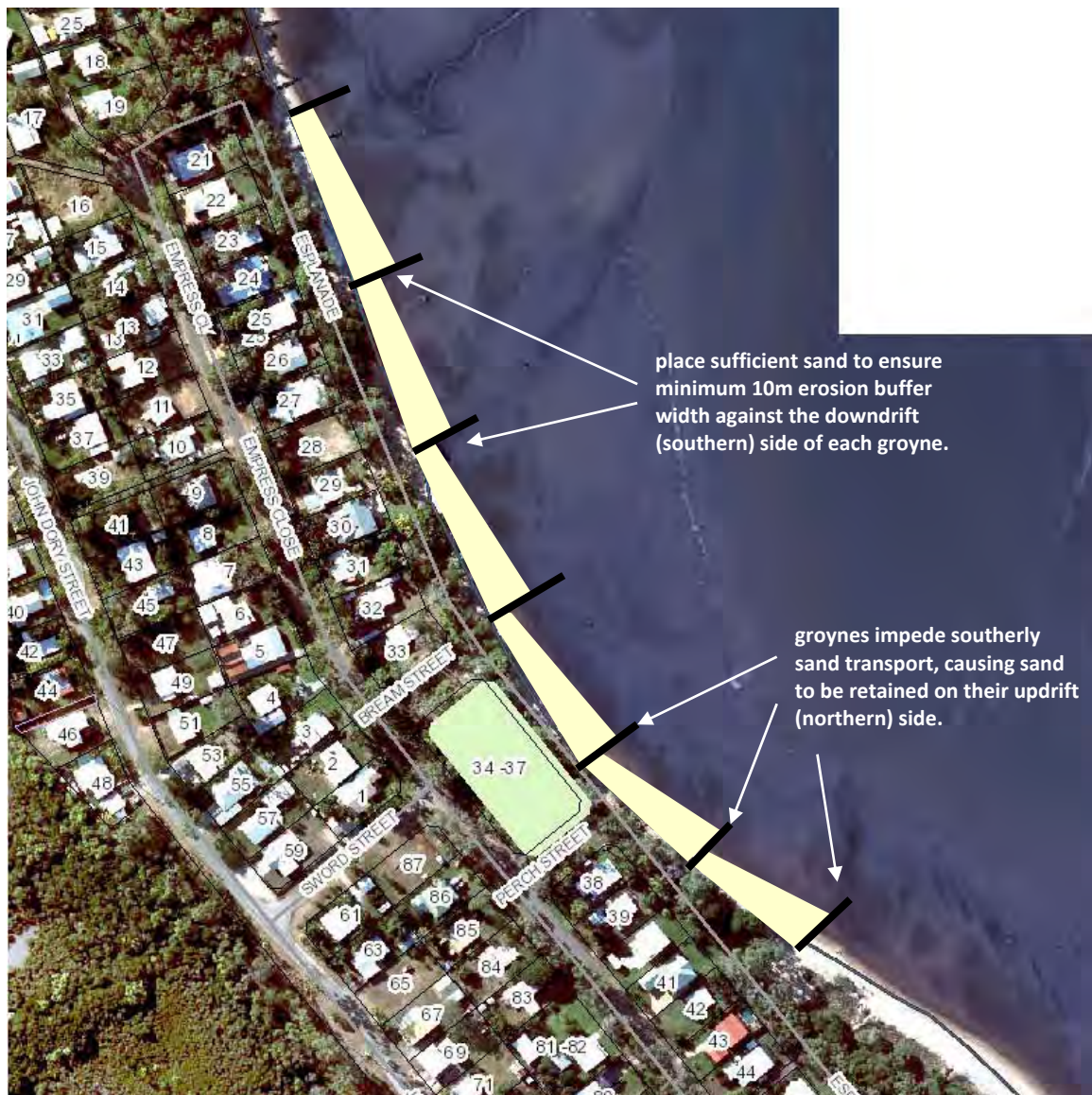
Figure 5.3 : Proposed groyne field to retain buffer
