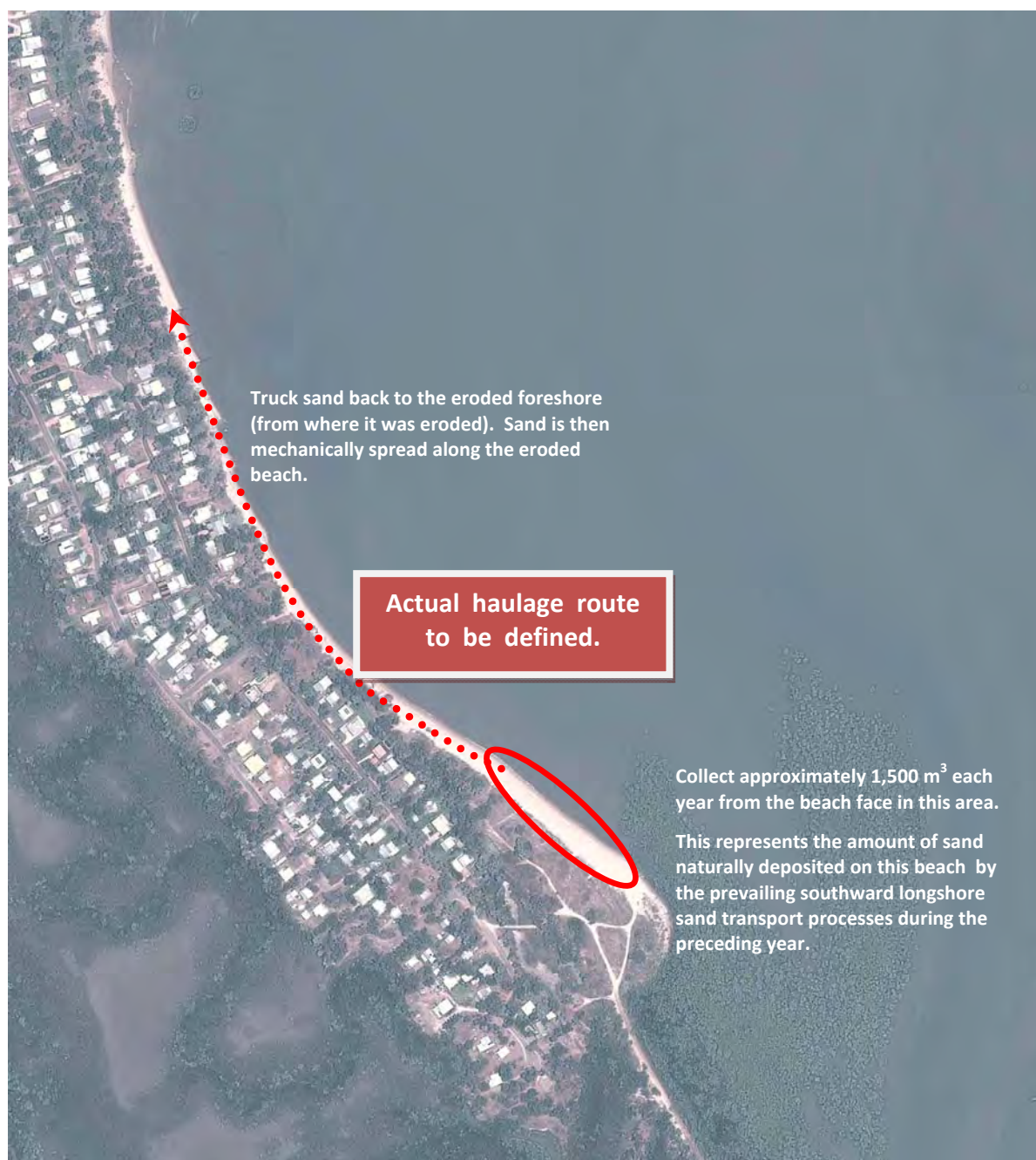
Figure 5.2 : Proposed back-passing of sand from southern accumulation area
