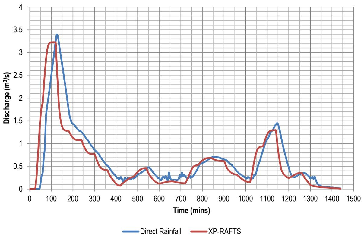
**Figure 2.1** Hydrology comparison for 'steep' test catchment
