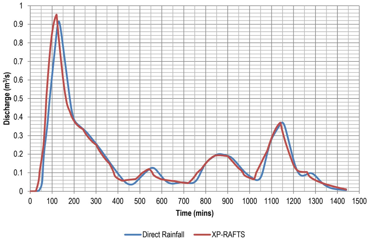
**Figure 2.2** Hydrology comparison for ‘flat’ test catchment
