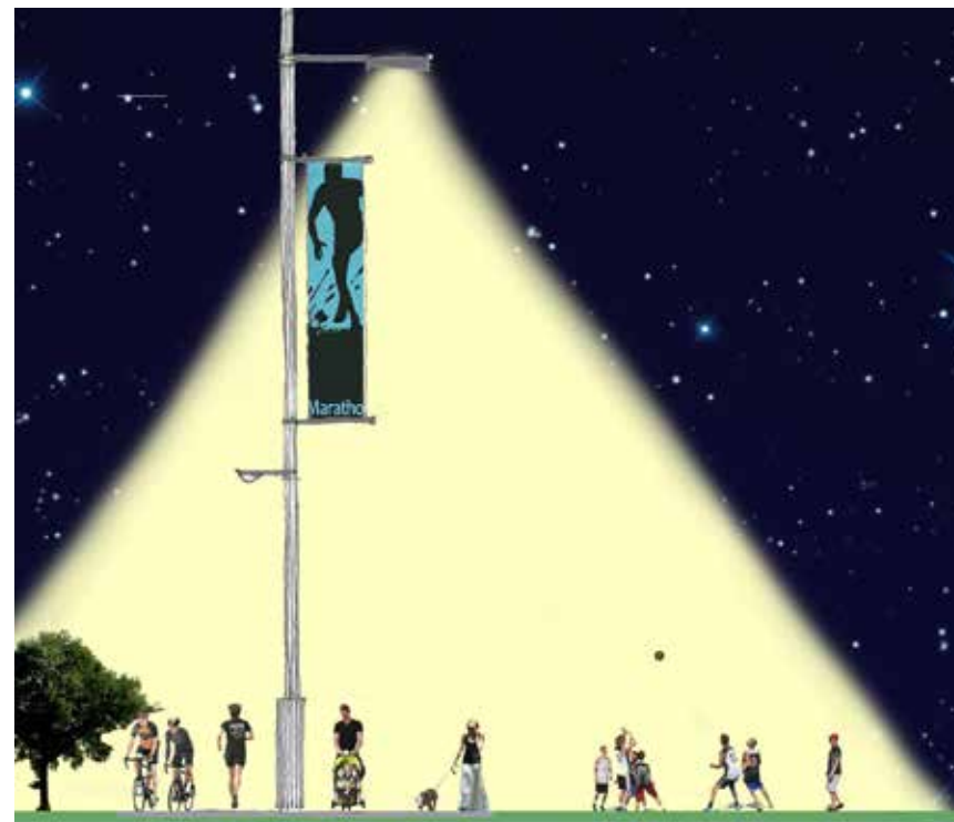
Figure 39: Demonstrates the lighting distribution given by a 10m smart pole, primarily utilised for open space and recreational or parkland areas
