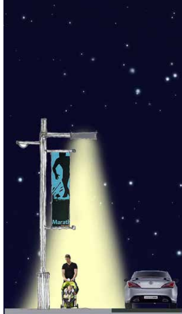
Figure 38: Exhibit the light distribution of the smart pole. Demonstrates a flat plate luminaire that will not detract from other features, while expressing a contemporary minimalist design approach
