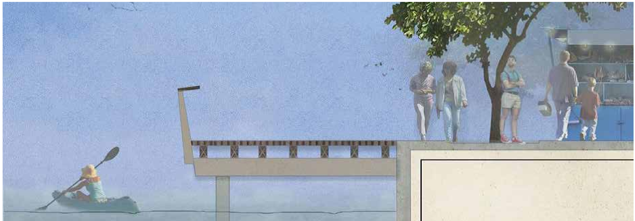
Figure 27: Type H - Wharf edge - vertical wall with concrete pavement behind and flush deck out over water
