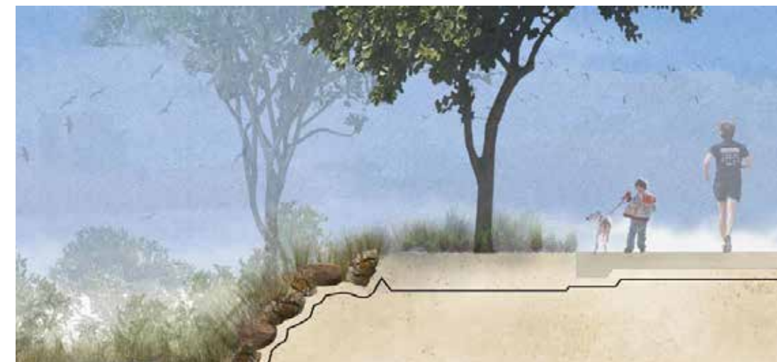
Figure 26: Type D - Rock batter with concrete path set back from top of batter with planted strip between
