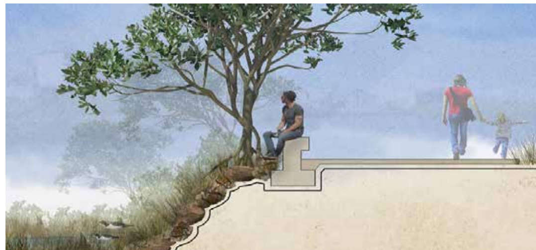
Figure 21: Type C – Rock batter with seating height concrete edge restraint to top of batter
