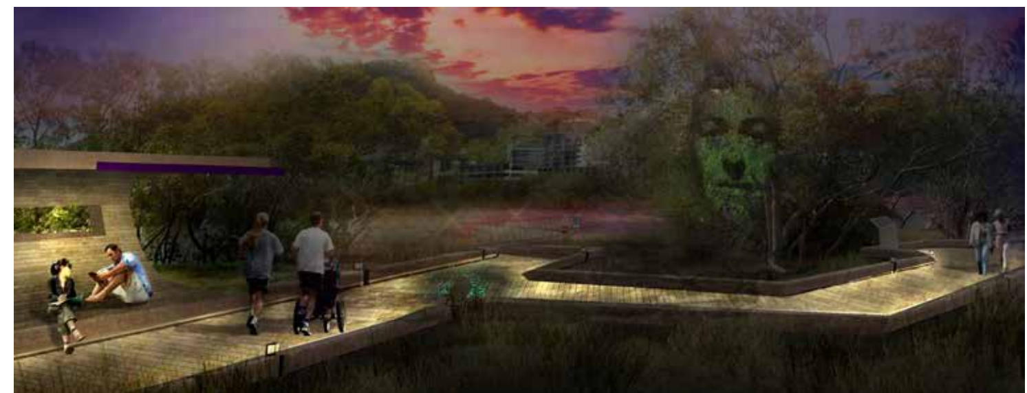
Figure 37: To optimise public safety it is important we aim for a vertical illuminance level and a uniform distribution of lighting and avoid creating dimly lit spaces between each light source. As demonstrated in the image above
