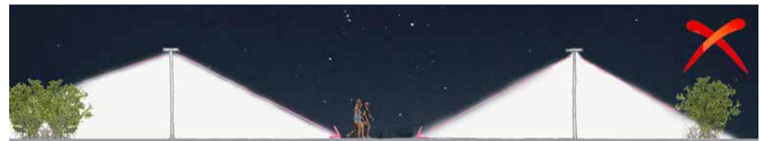
Figure 37: To optimise public safety it is important we aim for a vertical illuminance level and a uniform distribution of lighting and avoid creating dimly lit spaces between each light source. As demonstrated in the image above
