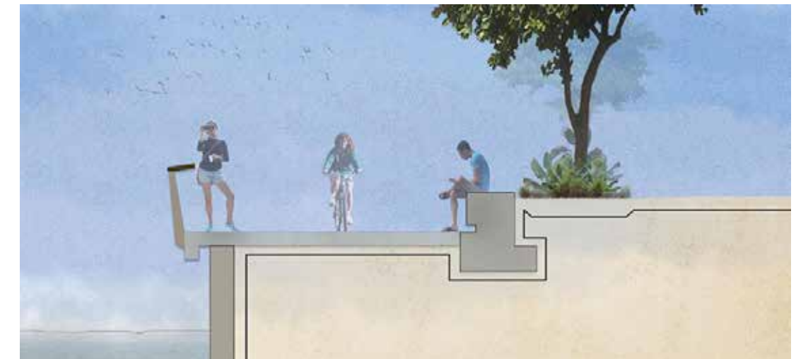
Figure 24: Type G – Wharf edge – vertical wall with concrete pavement interface
