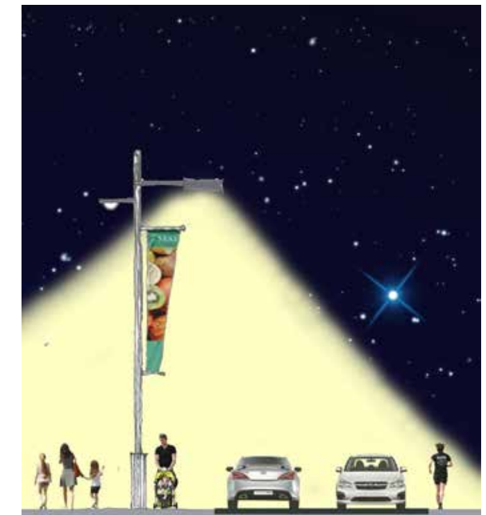
Figure 40: Exhibit the light distribution of the smart pole. Represents the light distributed by a 4-5m smart pole used primarily for to provide lighting for pedestrian areas. While Figure 22 displays the lighting provided by a 6-7m smart pole primarily used for lighting bridges, larger pedestrian areas and roadways
