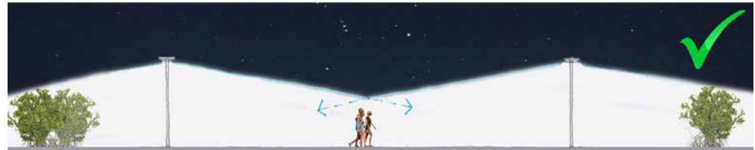
Figure 36: The overlapping of amenity light shown above will assist in providing the appropriate vertical lighting levels required for passive surveillance and a sense of security to patrons using the Townsville Waterfront
