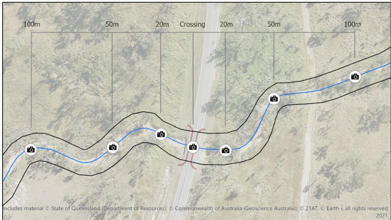
Figure 1. Standard locations along a waterway for fish habitat assessment. Where possible, a photo should be taken both upstream and downstream at each location. These distances are a starting point only and individual sites may require an assessment beyond these recommended distances
