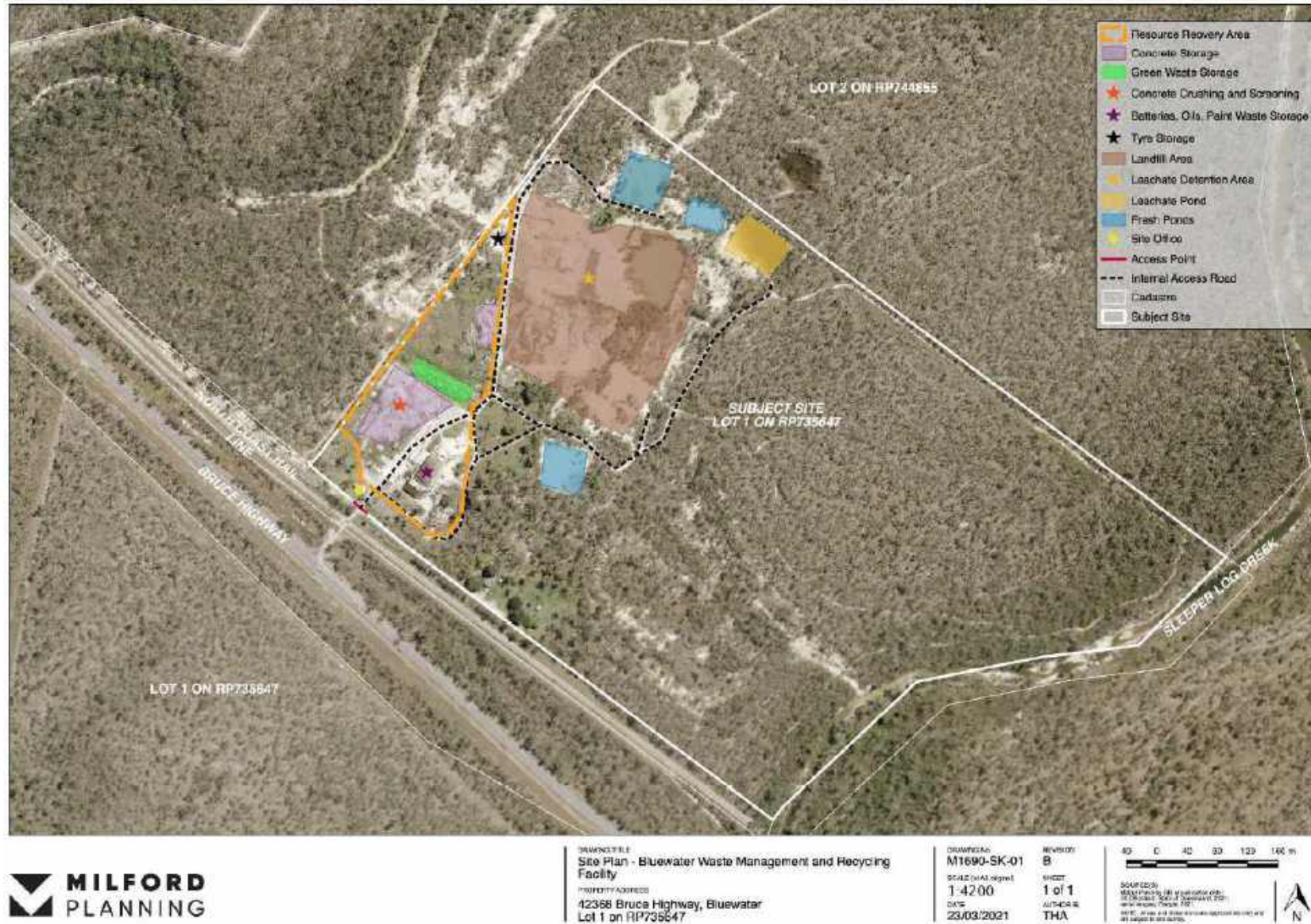
Figure 1: Current Site Plan with Waste Storage Locations
