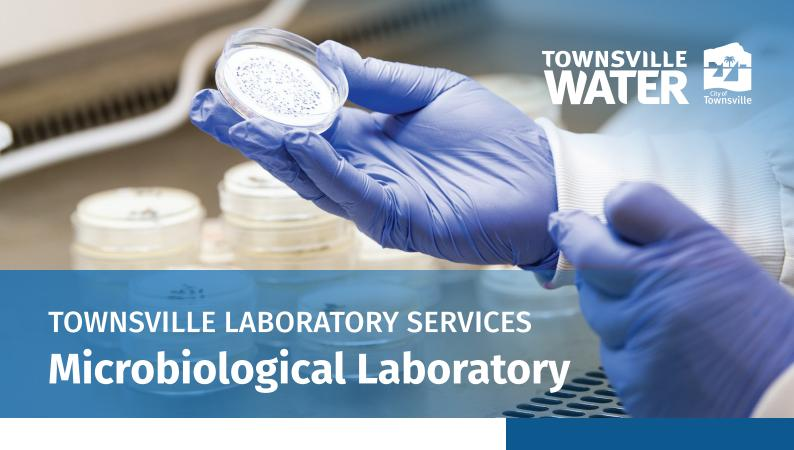
Townsville Laboratory Services (TLS) is nationally recognised for microbiological testing, using membrane filtration and differential media for most testing methods.
