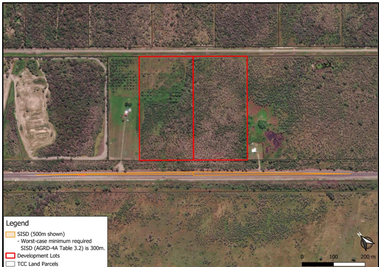
Figure 2-2 Safe intersection sight distances
