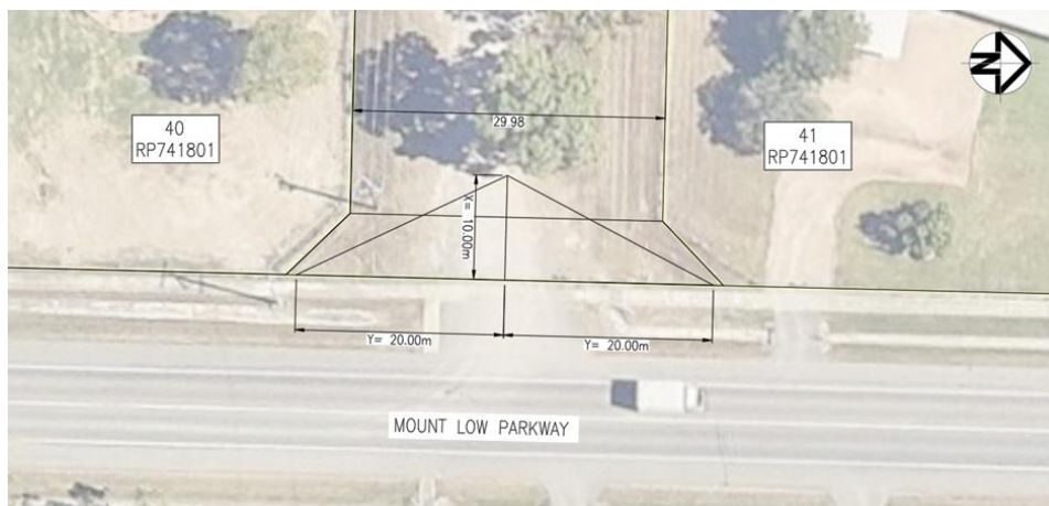
Figure 1. Available "X" (Driver's Sight Line into Property) and "Y" (SSD for the path users) dimensions at Access Intersection.
