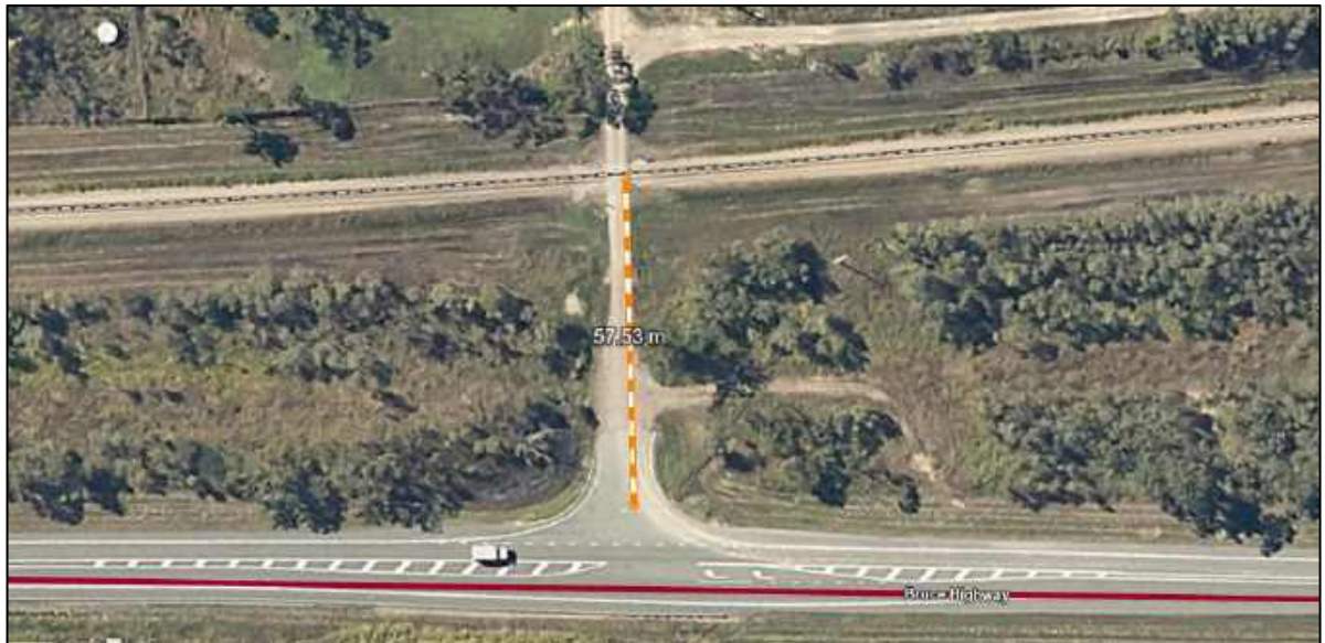
Figure 15. Available distance between intersection give way line and railway track
