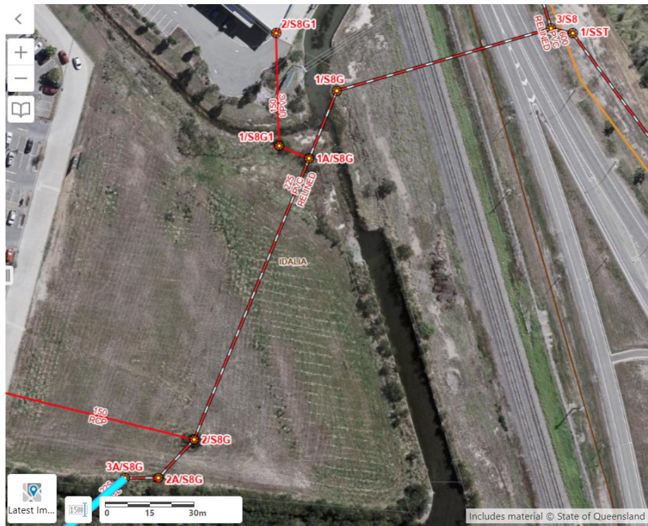
Figure 4.3 – DN225 Sewer between Bruce Hwy and Abbott St
