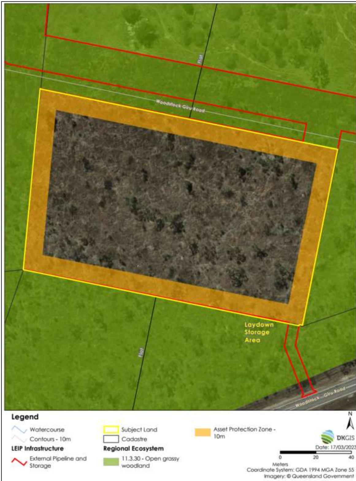
Figure 26: Minimum required APZ for BAL-40 (40kW/m<sup>2</sup>) – Laydown Storage Area
