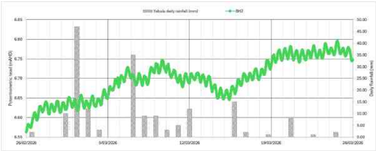
Figure 3.7 Daily rainfall (Yabulu Qld Nickel weather station: ID 32050) and logged potentiometric head at BL-BH2
