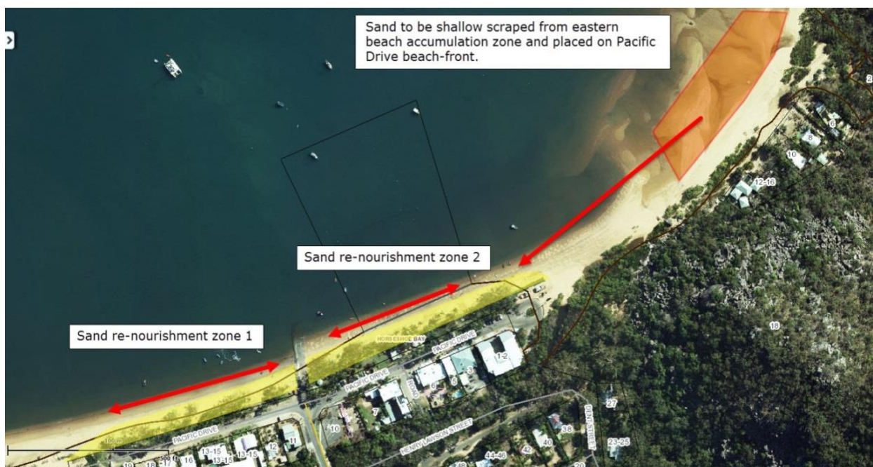
FIGURE 5-1 SCHEMATIC OF CURRENT SAND SCRAPING WORKS
