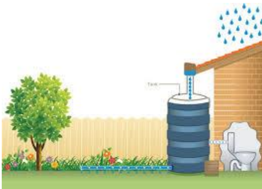
FIGURE 5-12 EXAMPLE OF A LEAKY TANK (SOURCE: WWW.STORMWATER.ASN.AU)
