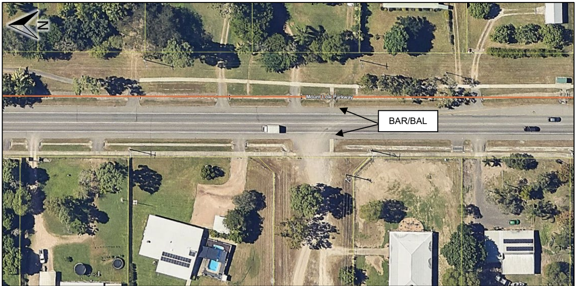
Figure 16. Current Turn Treatment.
