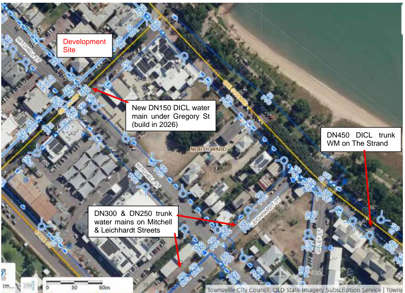
Figure 3.1 – Existing Water Mains
