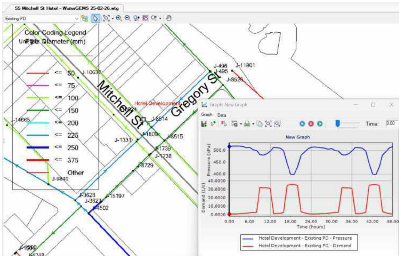
Figure 3.5 – 30 l/s Fire Flow Water Demand & Pressures
