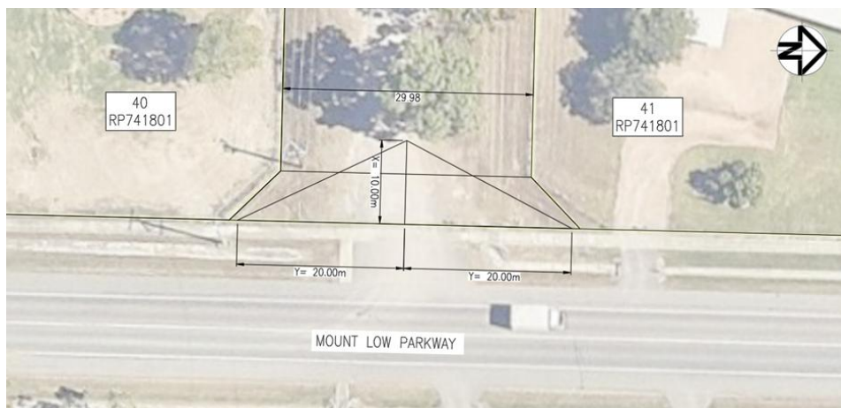
Figure 1. Available "X" (Driver's Sight Line into Property) and "Y" (SSD for the path users) dimensions at Access Intersection.
