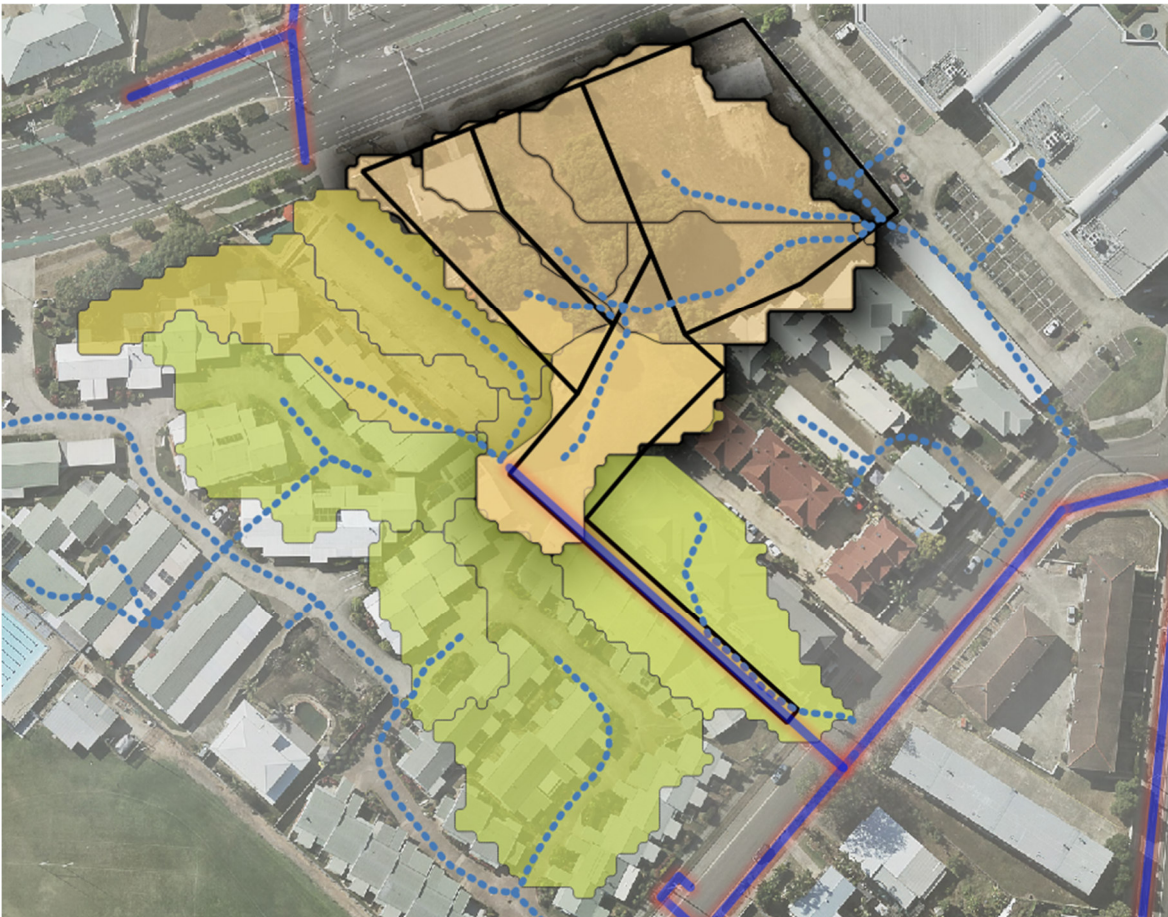
Figure 2 Catchments and flowpaths (solid blue lines indicate existing pipe network, dashed blue lines indicate overland drainage flowpaths).
