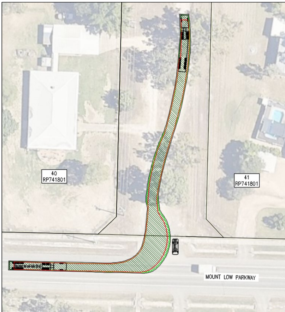
Figure 22. Semi-Trailer left turning into the Access/ B99 vehicle left turning out to South Mount Low Parkway.
