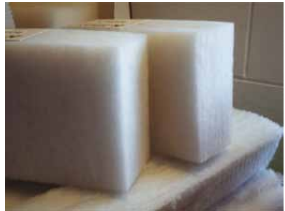
Figure 8 Example of bulk insulation (Photo: TCC).
