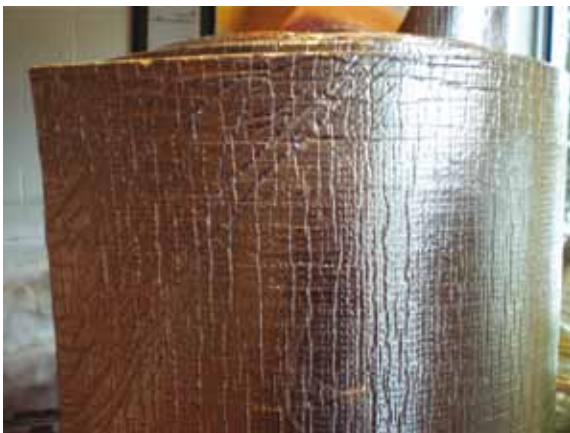
Figure 7 Example of reflective insulation (Photo: TCC).
