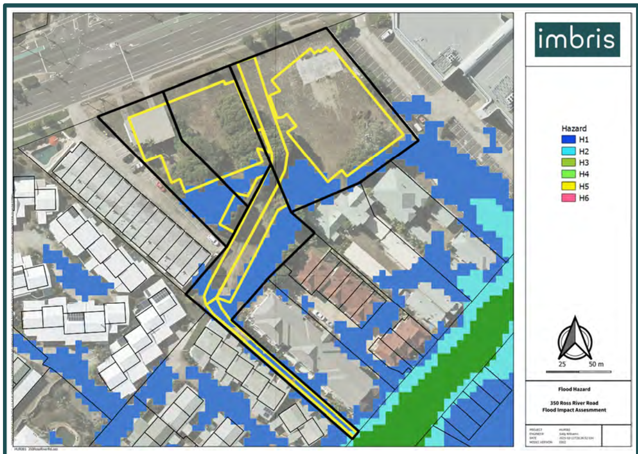
Figure 6 Developed Case 1% AEP Flood Hazard Mapping
