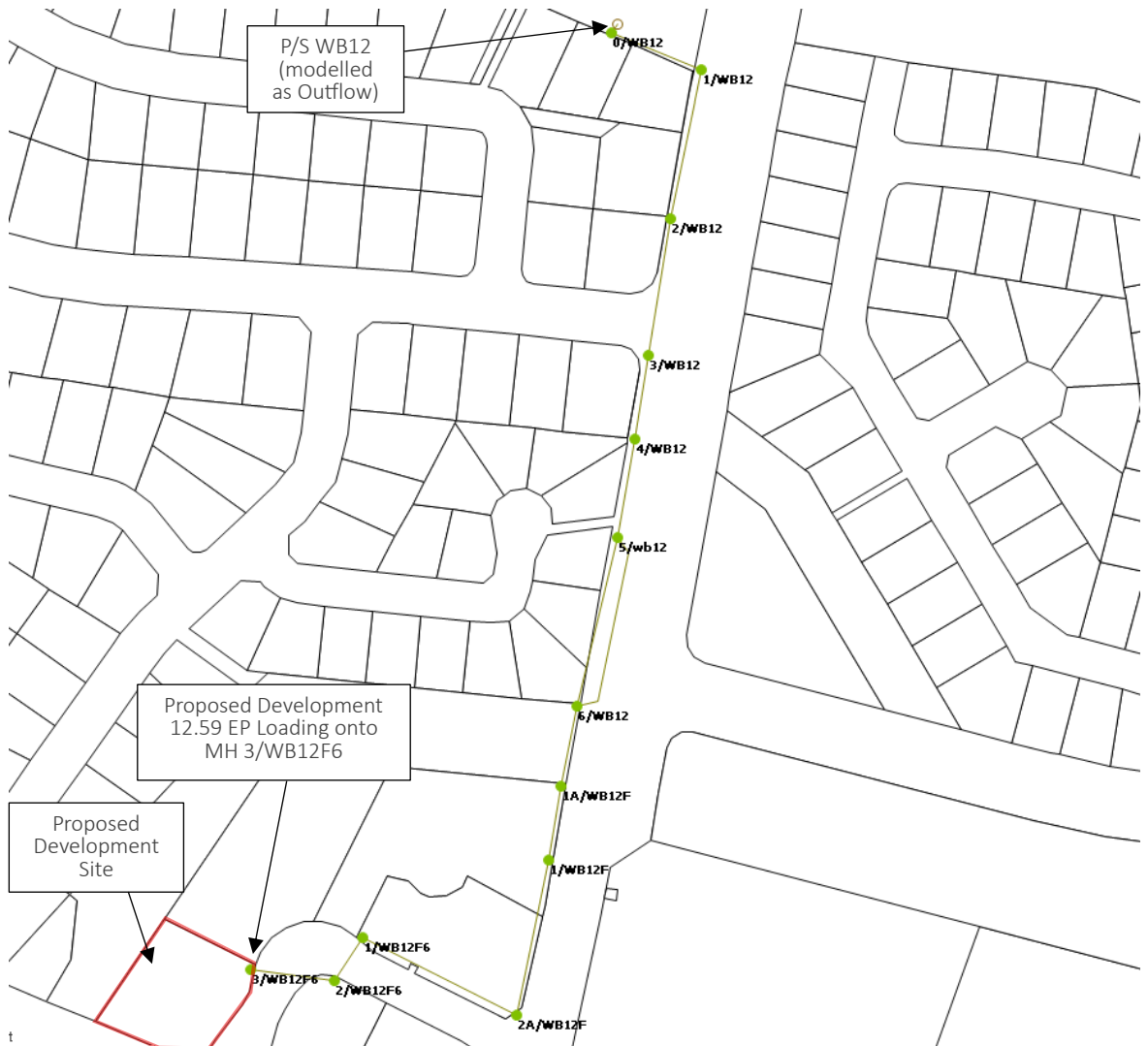
Figure 7: Hydraulic Model Screenshot – Modelled Sewer Gravity Main from MH 3/WB12F6 to P/S WB12
