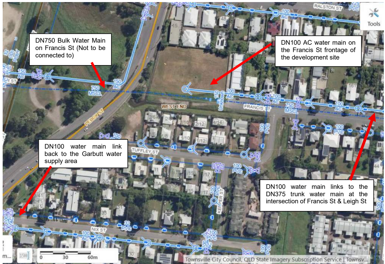
Figure 3.1 – Council GIS Plot of Water Network
