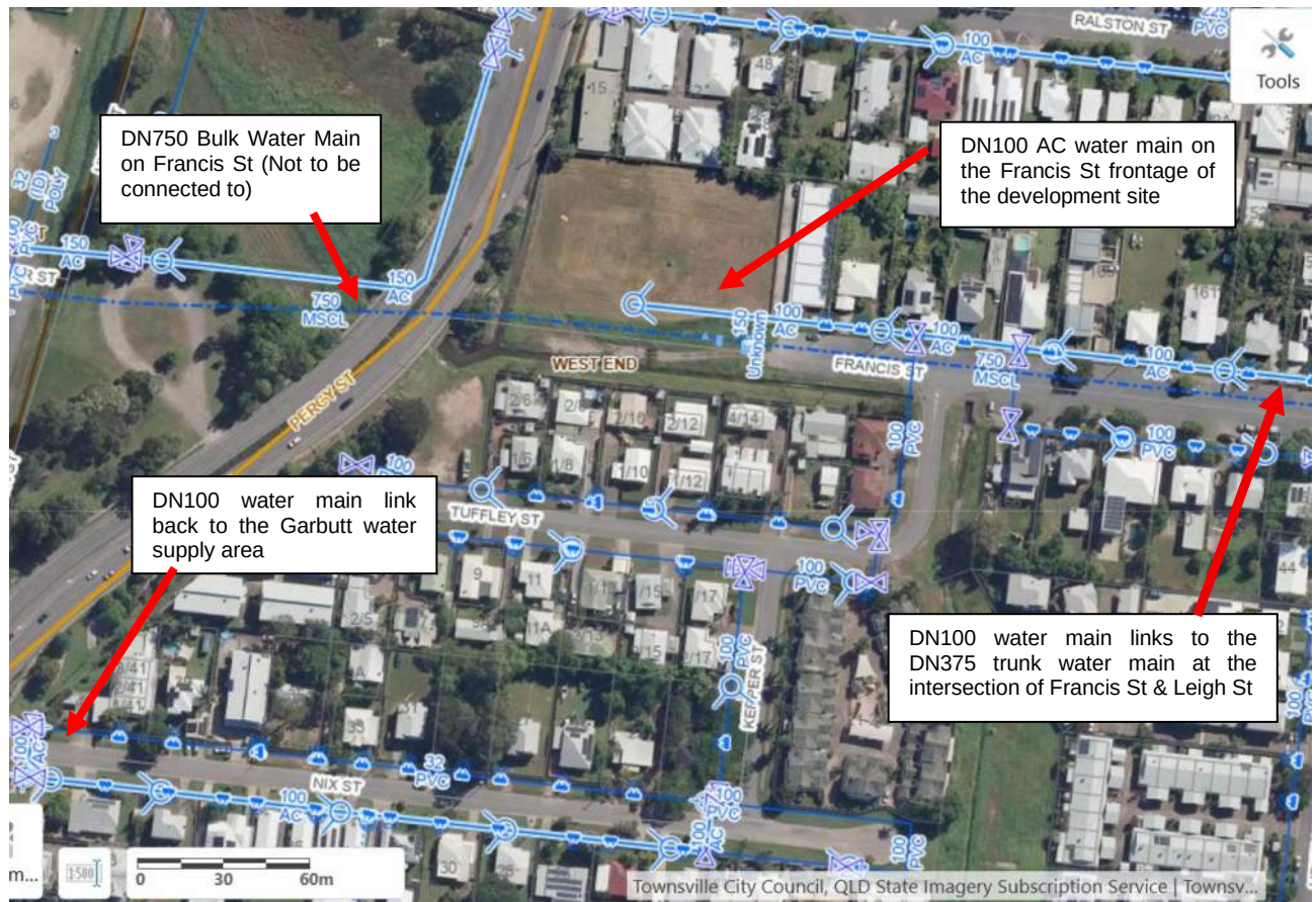
Figure 3.1 – Council GIS Plot of Water Network
