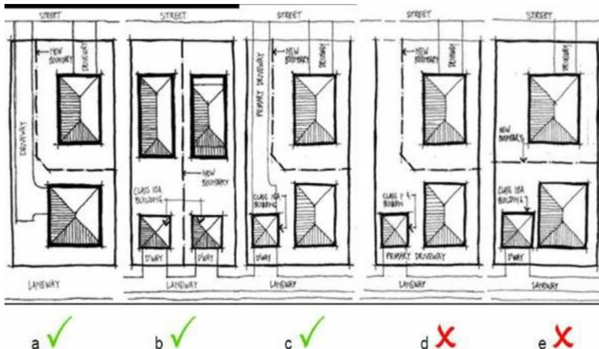
Figure SC6.4.3.16.2 Unacceptable and acceptable lot reconfiguration and access for properties adjacent to rear lane
