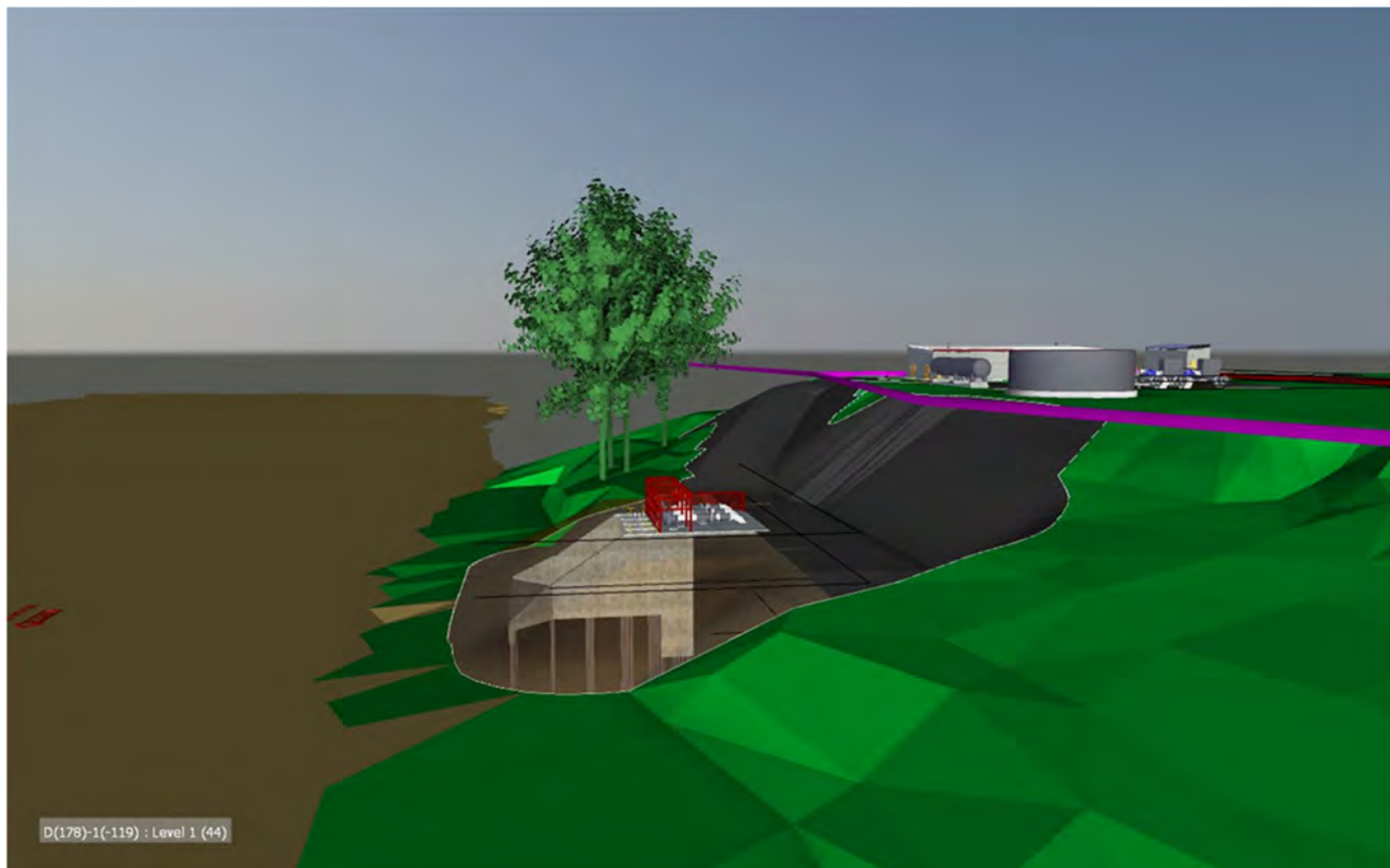
Figure 2.5 HPS2 Pump Station perspective and location relative to the existing upstream Sunwater Tom Fenwick Pump Station
