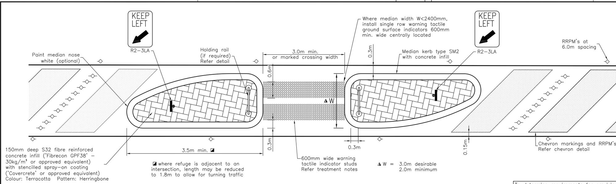
150mm deep S32 fibre reinforced concrete infill ('Fibrecon GPF38' - 30kg/m<sup>3</sup> or approved equivalent) with stencilled spray-on coating ('Covercrete' or approved equivalent) Colour: Terracotta Pattern: Herringbone
