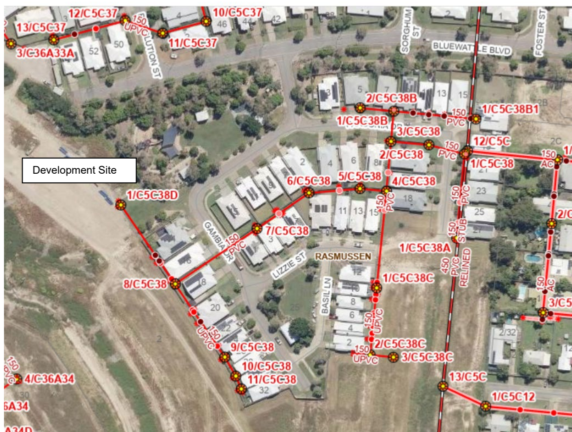
Figure 4.2 – Council GIS Extract of Existing Sewer System
