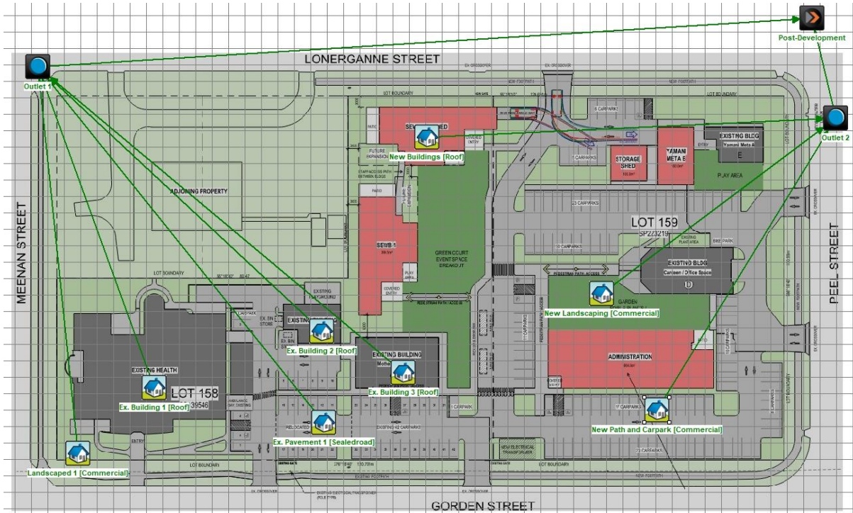
Figure 3 – MUSIC treatment train model of post-developed site with no treatment measures installed
