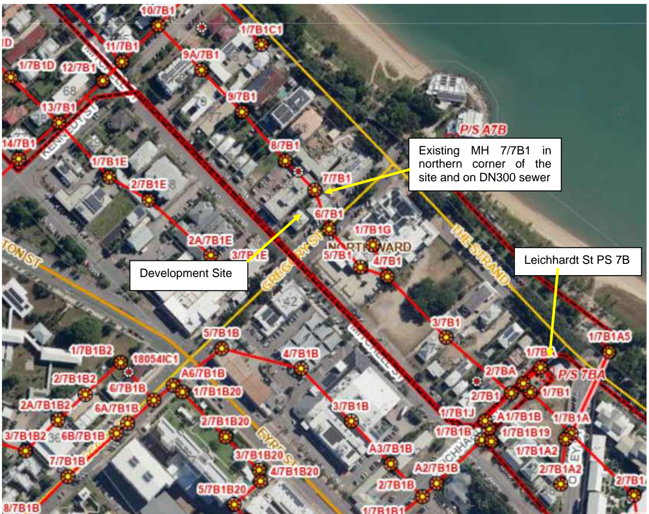
Figure 4.1 – Existing Gravity Sewer System
