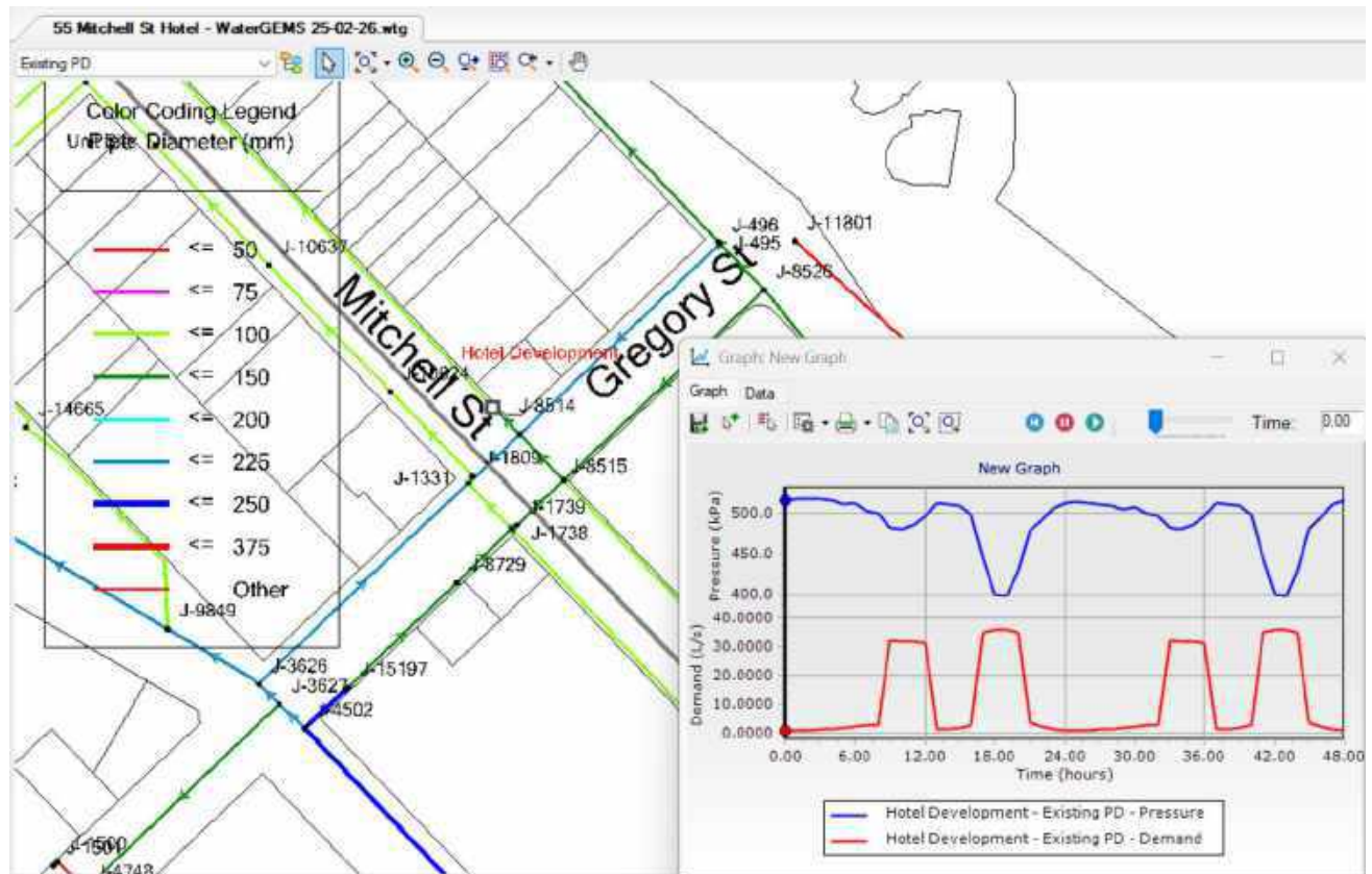
Figure 3.5 – 30 l/s Fire Flow Water Demand & Pressures
