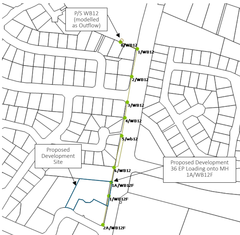
Figure 7: Hydraulic Model Screenshot – Modelled Sewer Gravity Main from MH 2A/WB12F to P/S WB12
