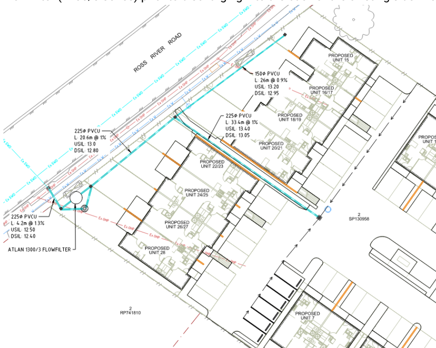
Figure 5.5 – Northern Catchment – Proposed Stormwater Drainage
