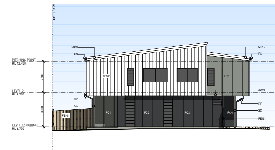
06 BLDG 08 WEST ELEVATION 1:100
