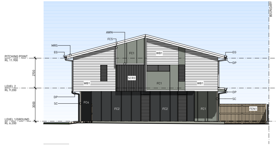
03 BLDG 04 SOUTH ELEVATION 1:100
