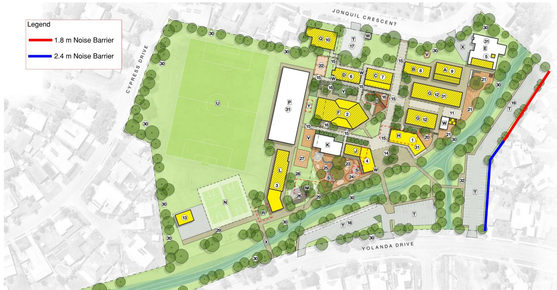
Figure 5 Recommended noise barriers
