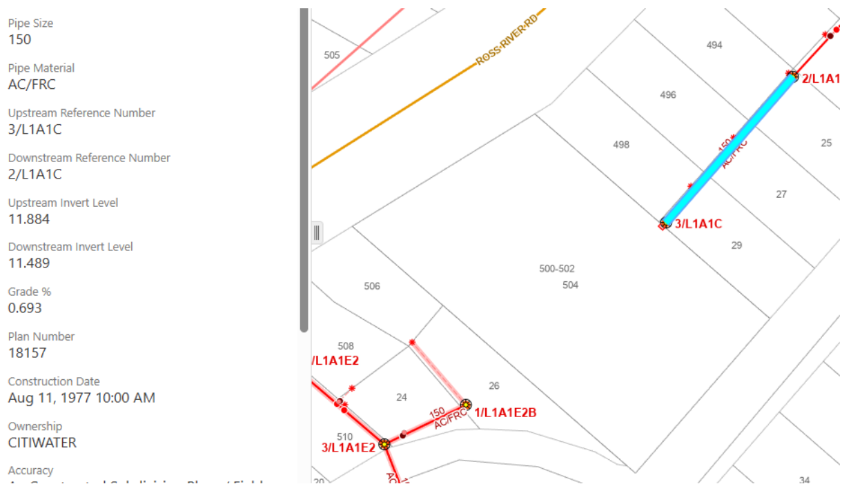
Figure 7.2 – TownsvilleMAPS existing sewerage layout
