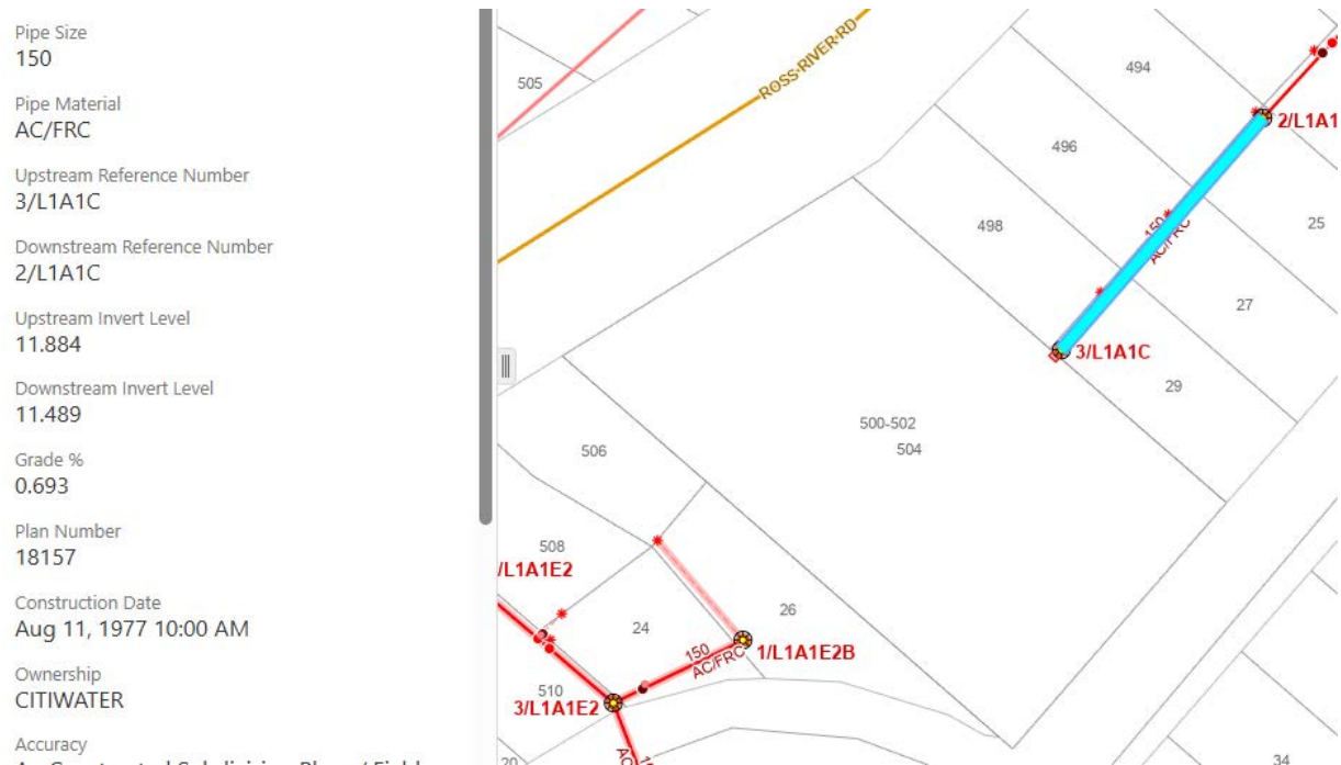
Figure 7.2 – TownsvilleMAPS existing sewerage layout
