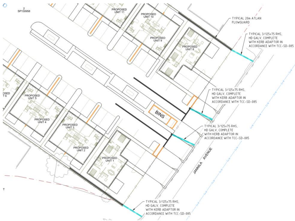
Figure 5.6 – Southern Catchment – Proposed Stormwater Drainage
