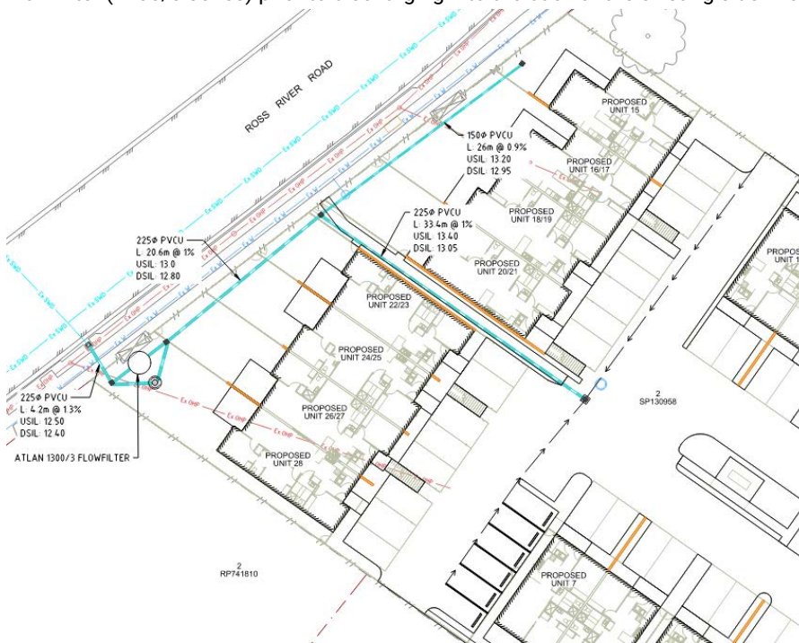
Figure 5.5 – Northern Catchment – Proposed Stormwater Drainage
