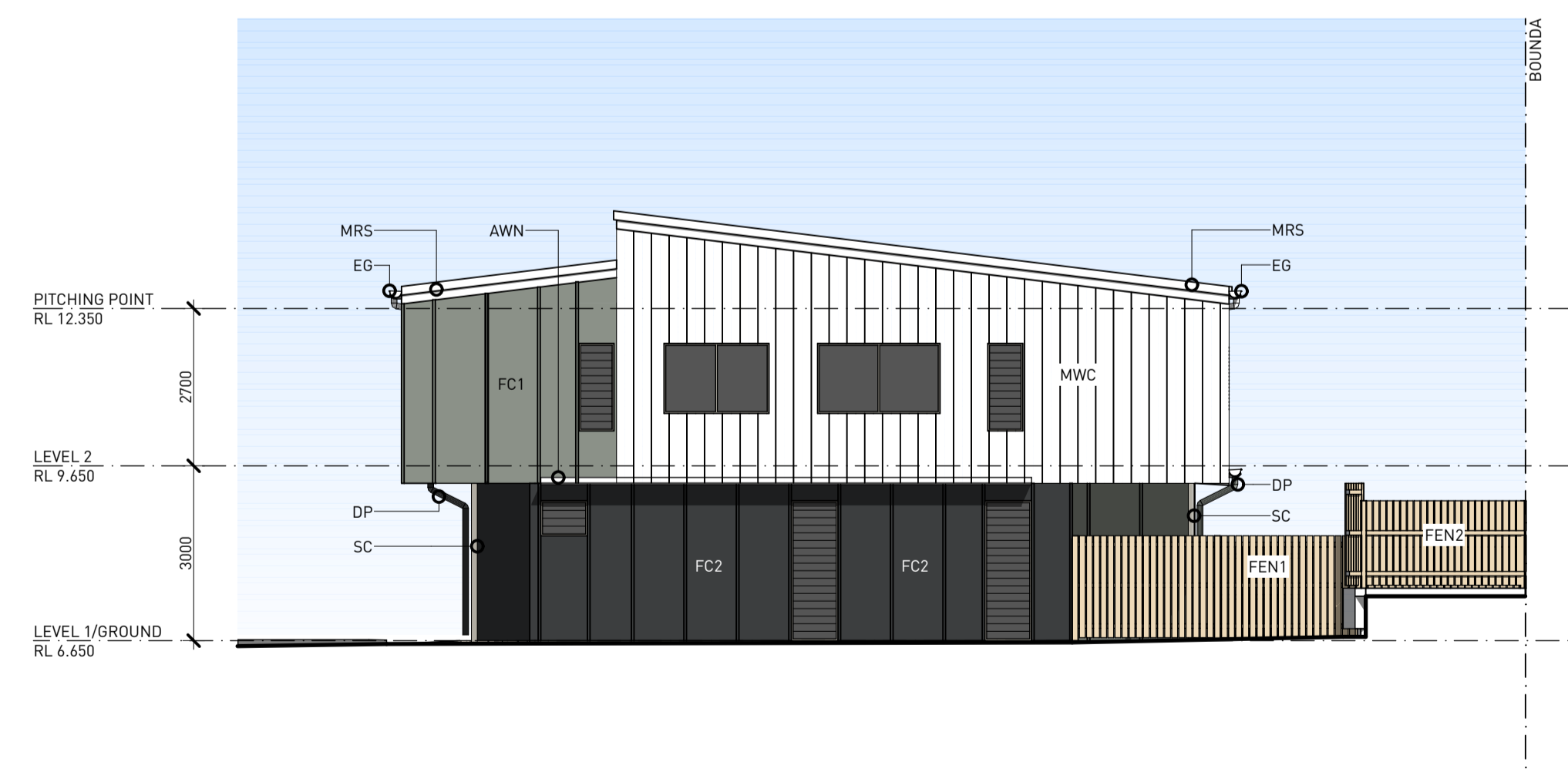
05 BLDG 02 WEST ELEVATION 1:100
