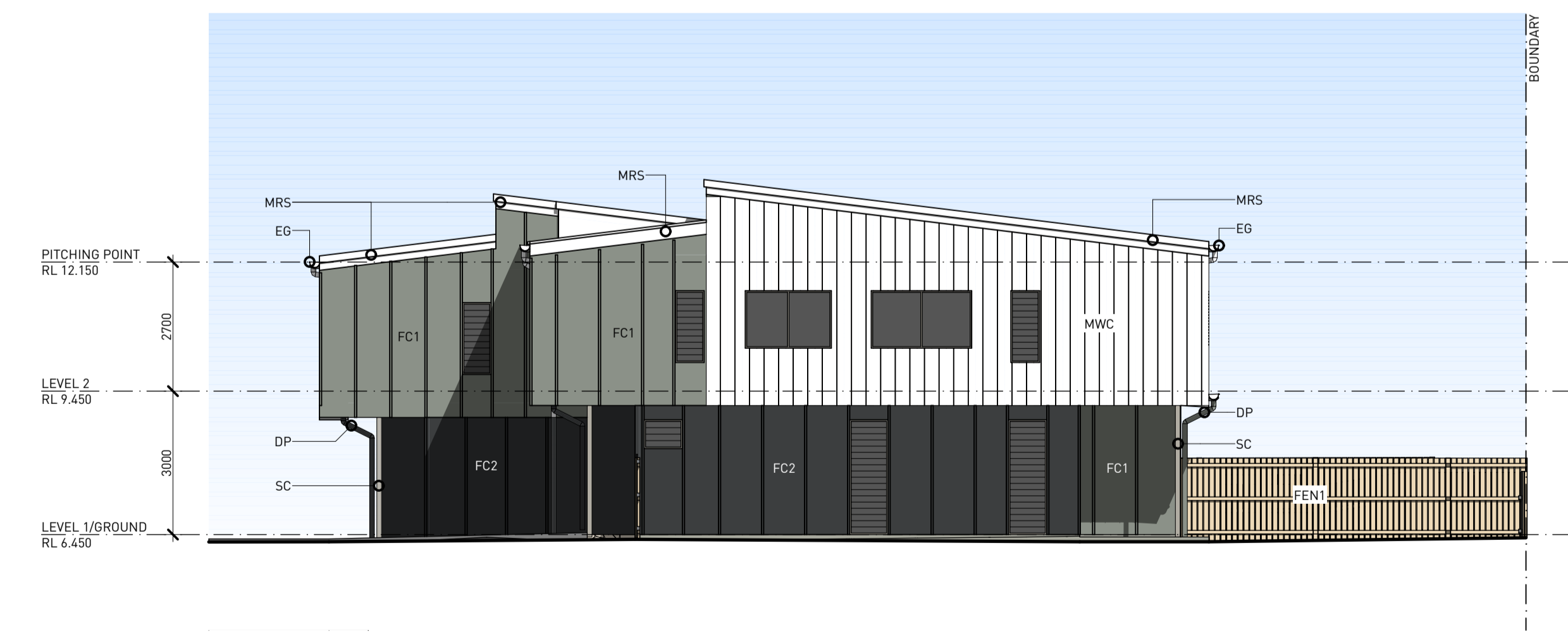
04 BLDG 03 WEST ELEVATION 1:100
