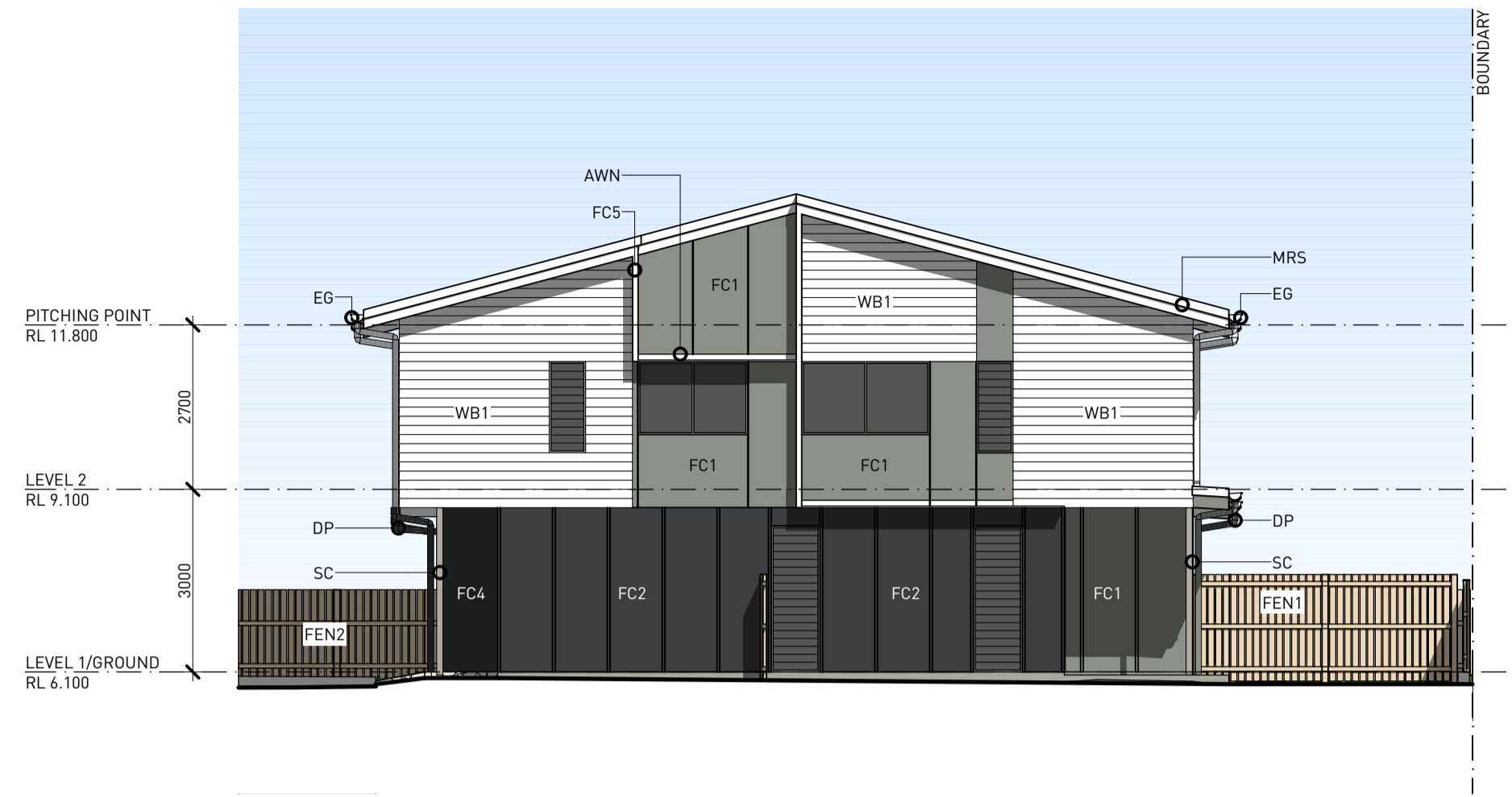
01 BLDG 05 SOUTH ELEVATION 1:100
