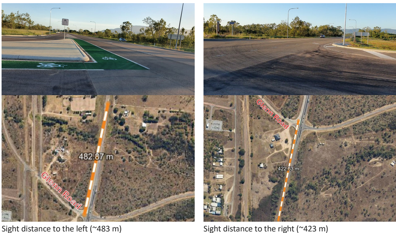
Figure 6.4 Sight distance to the left and right from Glenn Road to Flinders Highway
