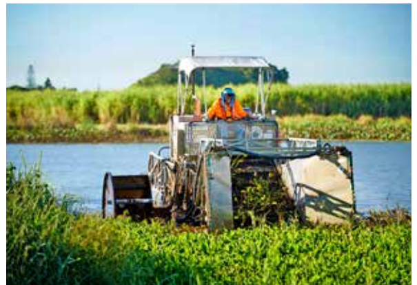
Taking action: water weeds officer using a weed harvester to remove aquatic weed in Lilliesmere Lagoon
