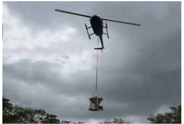
Aerial baiting: one control option includes using a helicopter with a 1080 bait disperser.
