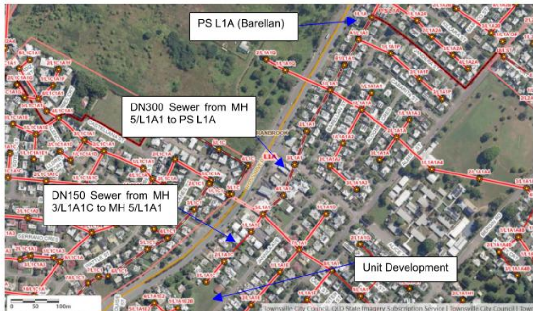
Figure 4.1 – GIS Plot of Existing Sewer System
