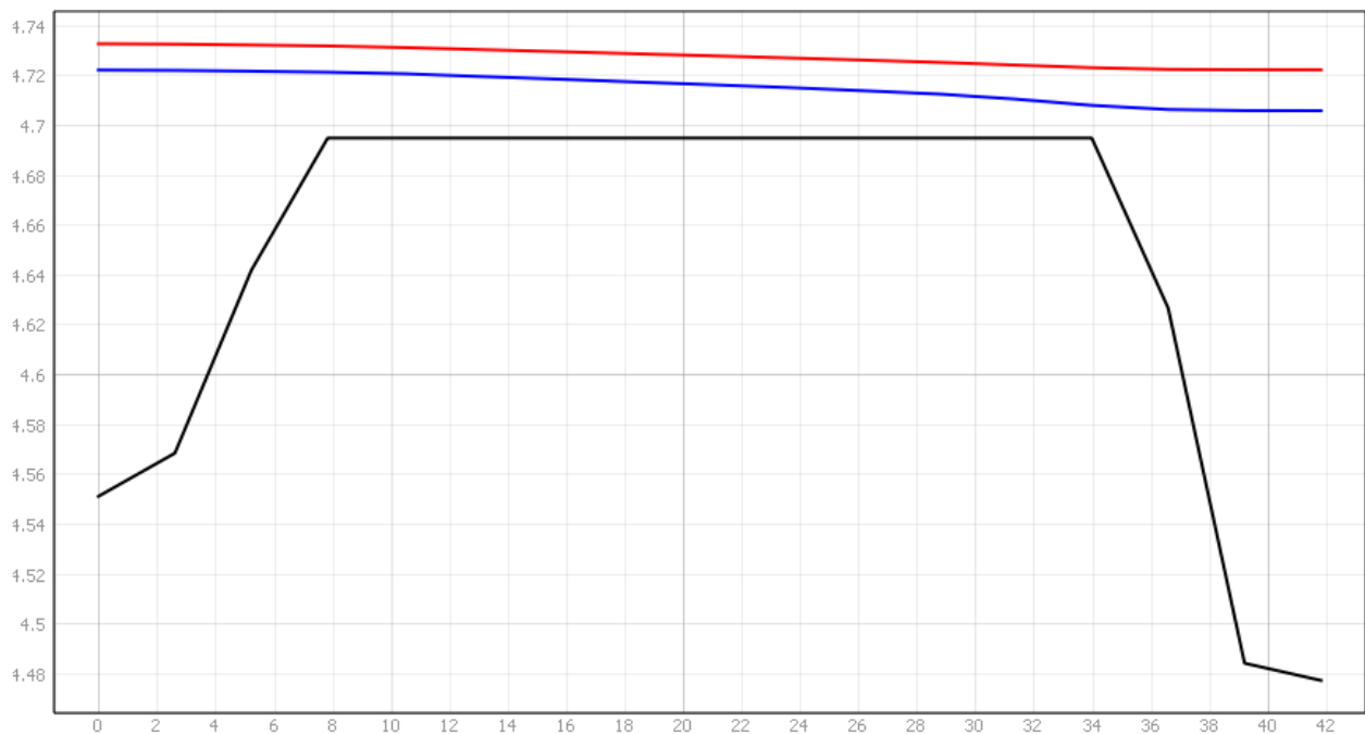
Figure 2 – Church floor level versus flood level (baseline WSL in blue, developed WSL in red)
