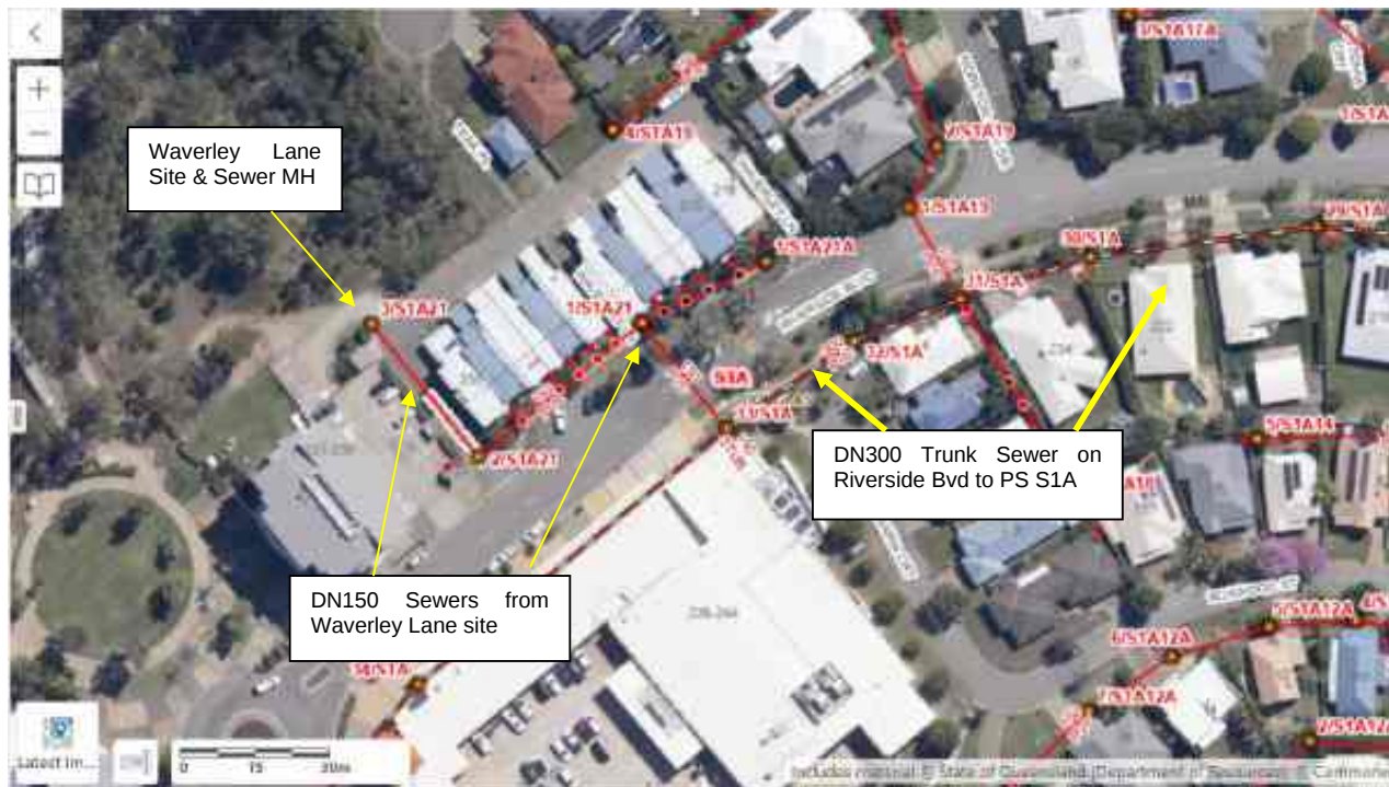
Figure 4.1 - Existing Sewer Infrastructure Figure
