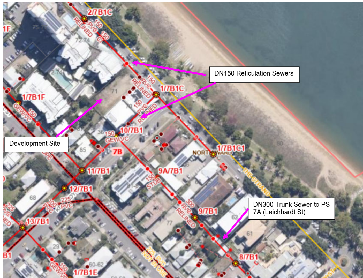
Figure 4.1 – GIS Plot of Existing Sewer System
