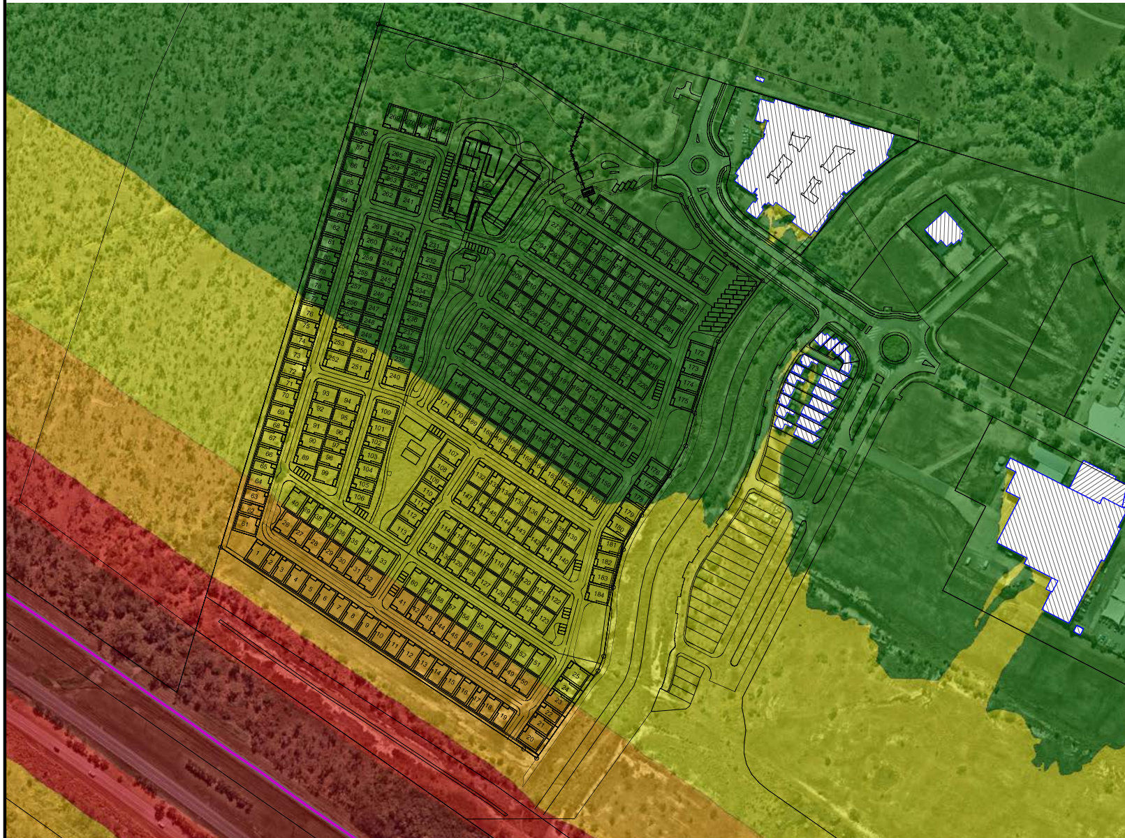
Figure 10 - Northshore LLC - Railway Noise Levels - First Floor Facade Corrected SEM Noise Contour Map at 4.6m Above the Ground Without Noise Barriers
