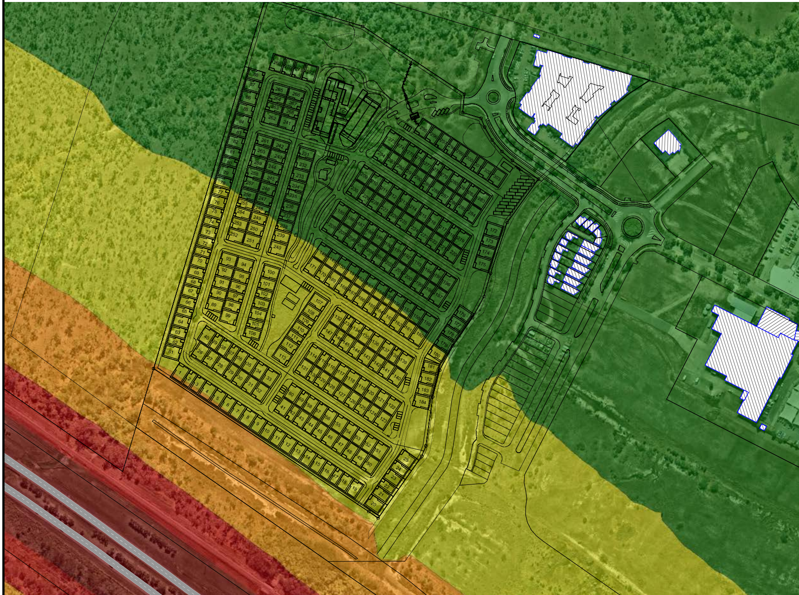
Figure 8 - Northshore LLC - 2046 Road Traffic Noise Levels - Facade Corrected L_{A10,18hr} First Floor Noise Contour Map at 4.6m Above the Ground Without Noise Barriers
