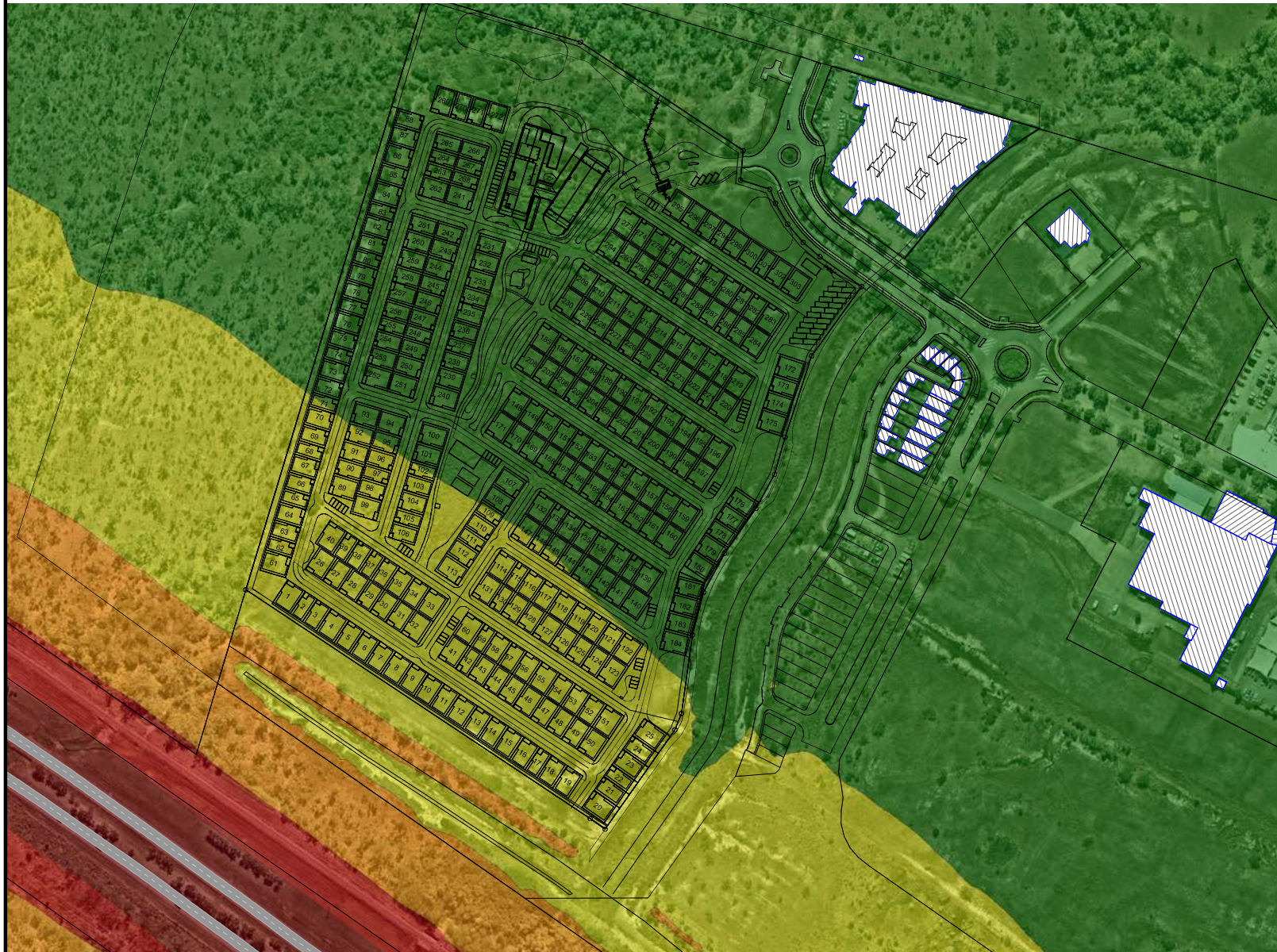
Figure 7 - Northshore LLC - 2046 Road Traffic Noise Levels - Facade Corrected L_{A10,18hr} Ground Floor Noise Contour Map at 1.8m Above the Ground Without Noise Barriers
