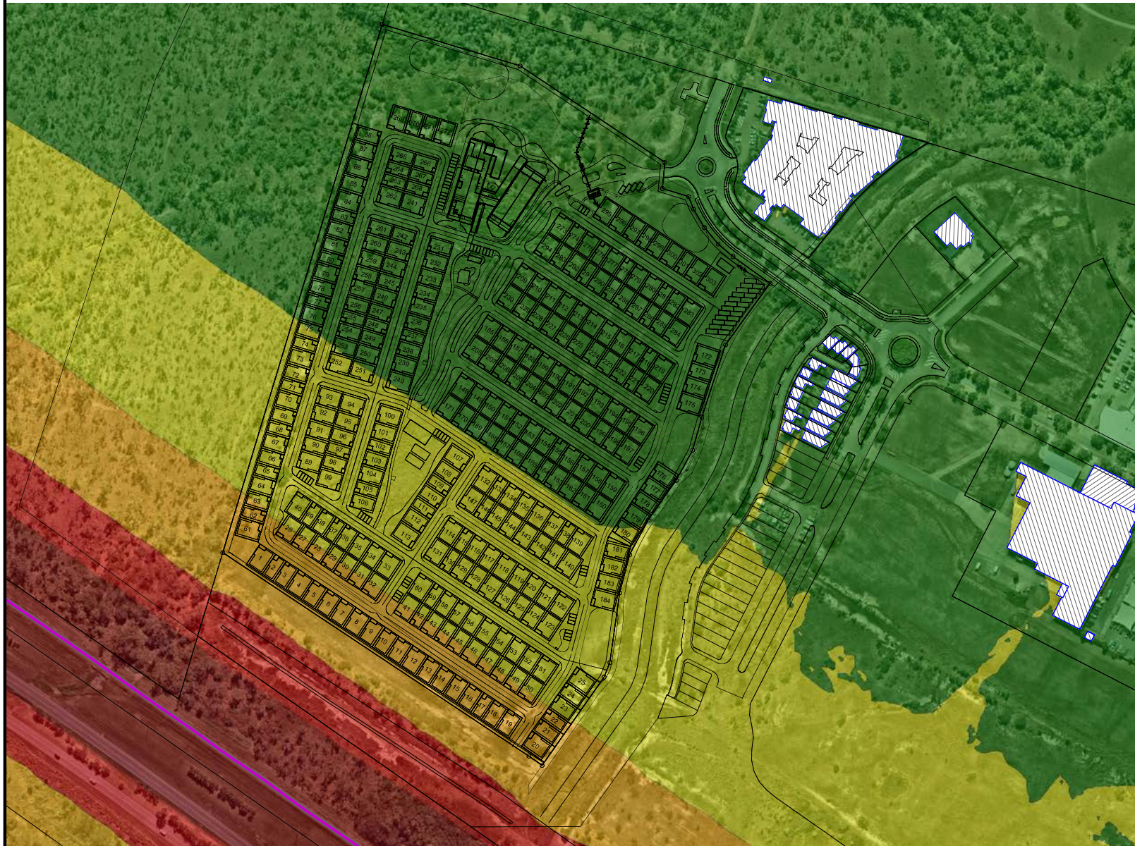
Figure 9 - Northshore LLC - Railway Noise Levels - Ground Floor Facade Corrected SEM Noise Contour Map at 1.8m Above the Ground Without Noise Barriers
