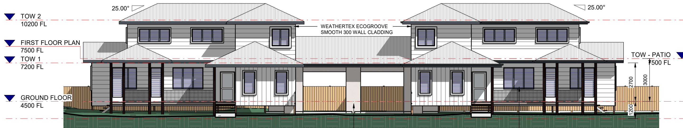
GRANITE STREET ELEVATION 1 : 125
